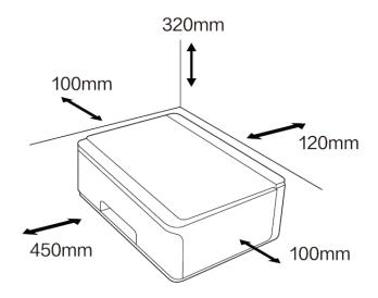
Please ensure that sufficient space is reserved to open the machine cover and feed tray.
