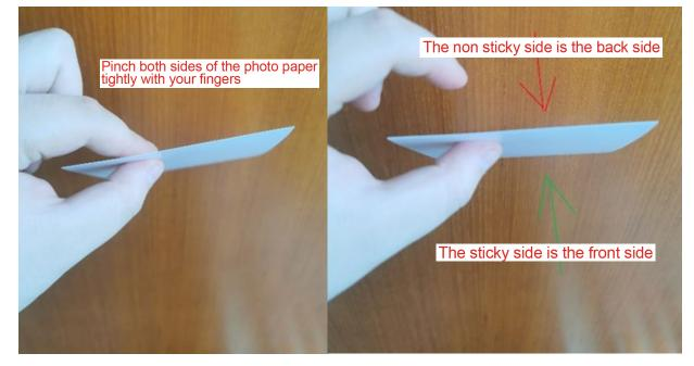
3. The photo paper is properly placed in the paper box; Make sure that the front of the photo paper is facing outwards (or upwards), and the back touches the baffle plate when it is put into the paper box. At the same time, adjust the blue plate in the paper box to clamp the photo paper correctly.
