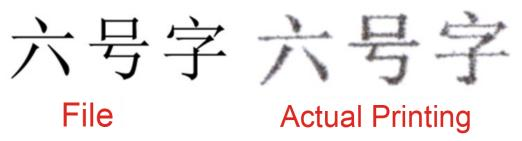
Causes: The original document is displayed in black on the display, while the laser printer uses black solid toner and the inkjet printer uses black water-based ink, which is lighter than the black color as printed by the laser printer and shown on the screen.
