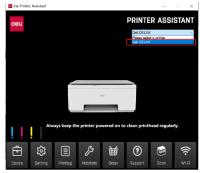
4. Select the connected printer from the drop-down list.
