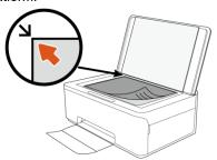
Load paper in the feed tray. Place the original printing face down near the icon in the upper left corner of the presentation platform. Press
